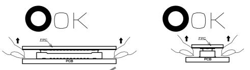
(2) If the connector council be un-mated parallel it can be removed diagonally from the pitch direction. Be careful to do so since this action applies stress on the contact.
