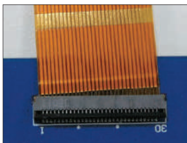
✗ Skewed FPC Insertion
