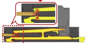
If the actuator is closed when the FPC is not inserted and then reopened, the contact gap becomes narrower.
