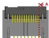
⇒ Contact supports the rotating axis of the actuator only in the upward direction
