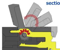
⇒ Contact covers the rotating axis of the actuator.
