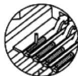
Uplift of the conductor
