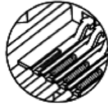
Insufficient amount of solder used
