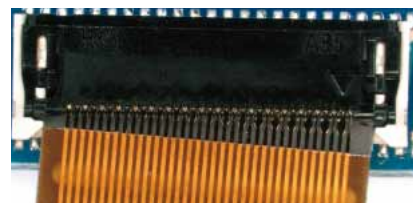
FPC is inserted diagonally.
