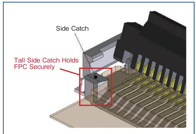
Lock Design Ensures High FPC/FFC Retention Force
