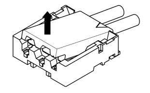
Dlift up to the upper direction and positive lock is released. Removal completes.
