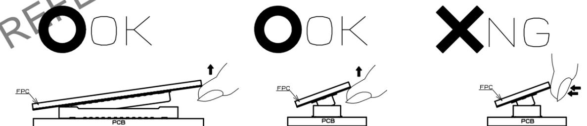
(3) IF THE FPC IS NOT RIGID, THE CONNECTOR CAN BE BROKEN. PLEASE CHECK THE ACTION OF THE FPC TO BE USED REPEATEDLY AT THE TIME OF TRIAL PRODUCTION. BE CAREFUL TO UN-MATE THEM FROM THE PITCH DIRECTION, PULLING IT FROM THE CORNER CAN ALSO RISK TO PUTTING STRESS ON CONTACTS.
