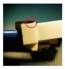
· Front edge of the retainer is touching to the crimp housing.
