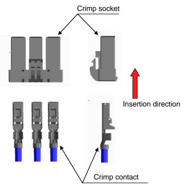
How to insert wire into multipole contact
