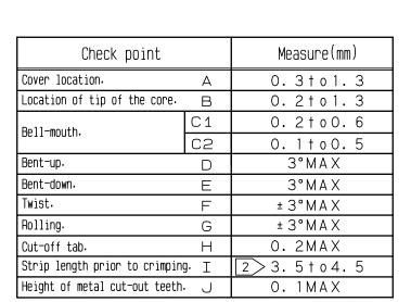
Note 1 To adjust applicator, please check the crimping condition (crimping height and configuration) by using cable.
