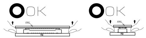
(≥) IF THE CONNECTOR CANNOT BE UN-MATED PARALLEL IT CAN BE REMOVED DIAGONALLY FROM THE PITCH DIRECTION. TO DO SO SINCE THIS ACTION APPLIES STRESS ON THE CONTACT.
