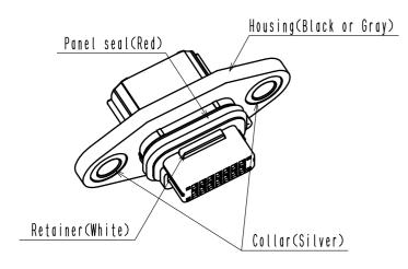
Please protect the panel seal not to be touched with other objects after insert the terminals and set the retainer. The protector is required not to be deformed excessively during packaging, shipping and being stored.
