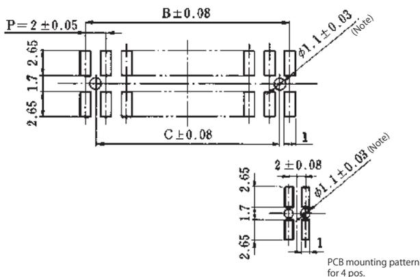
Note : The connector positioning boss is a structure that is lightly press-fitted into the board hole. When mounting on the board, press the connector lightly from above to make sure that the positioning boss is inserted securely into the board hole and that the connector leads are not floating off the board. For automatic board placement, recommended boss dia. is  $\phi 1.2 \pm 0.1$ .
