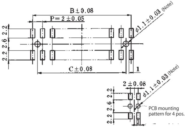
Note : The connector positioning boss is a structure that is lightly press-fitted into the board hole. When mounting on the board, press the connector lightly from above to make sure that the positioning boss is inserted securely into the board hole and that the connector leads are not floating off the board. For automatic board placement, recommended boss dia. is  $\phi 1.2 \pm_{0}^{0.1}$ .
