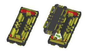
2. Once aligned, the connector engages. You can feel the mated height of the connector lower.
