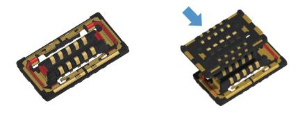
2. Once aligned, the connector engages. You can feel the mated height of the connector lower.
