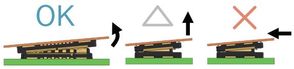
3. If the FPC does not have sufficient rigidity, solder stripping or connector breakage may occur. Please use it after checking the repetitive operation with a flexible board in advance, such as during a trial manufacture run.
