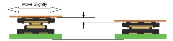
4. Check that mating is completed. If one side is floating, or if it is mated at a diagonal, remove and re-mate.
