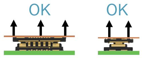
2. If difficult to remove, extract the connector diagonally in the direction of the pitch. Note that removal from the widthwise side will apply a large load to the contacts. When removing from the width direction, pull the end of the FPC in the upward direction. (When a force is applied in the horizontal direction, a large load is applied to the contact.)
