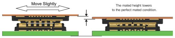
3. In the engaged state, the connectors are parallel to each other, and the connectors cannot move forward, backward, left, or right. Complete mating from this state.
