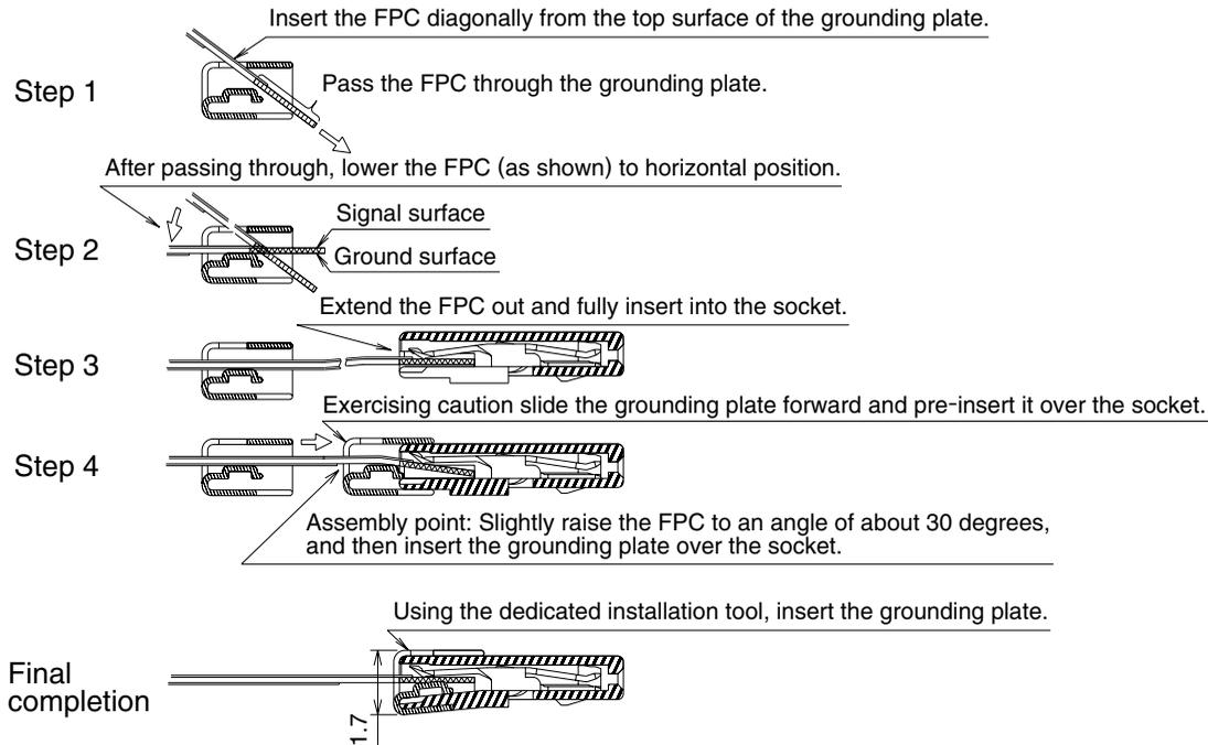
Note 1: The grounding plate and the plug are supplied as separate components.
