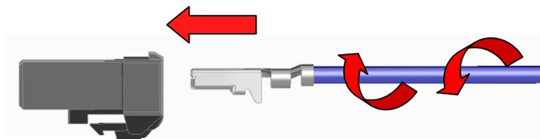
Twisting wire may deform the contact or crimp socket. Please Insert the contact without twisting wire.
