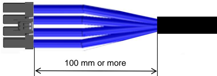
When using a multipole terminal, be aware that the strip length for the outside cables should be longer to provide it with a flexion portion, as well as to not apply any load such as excessive torsion.
