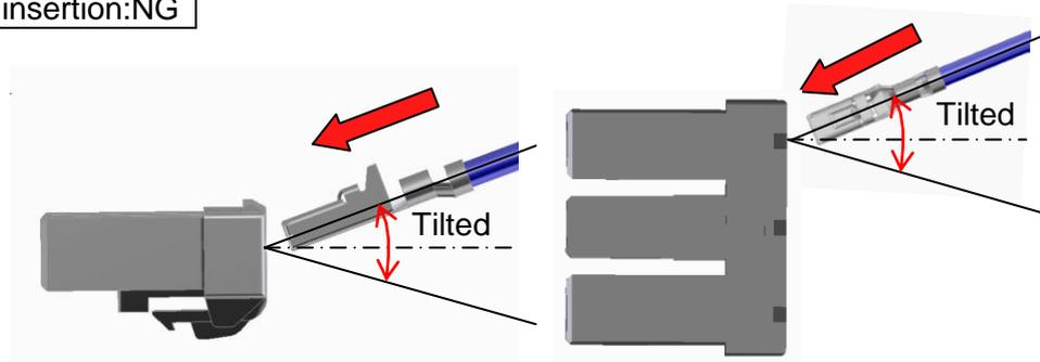
Insertion with tilted angle may deform the contact or crimp socket. Please Insert the contact without tilted.
