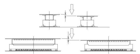
3) Once aligned, the connector pair does not move back and forth and around as they are located in a parallel position. Mate the connectors completely by applying force in this condition. We recommend to push the connector with two fingers for 50 pins or more to press down the whole connector evenly. One end might not be inserted enough to result in half mating for high pin counts.
