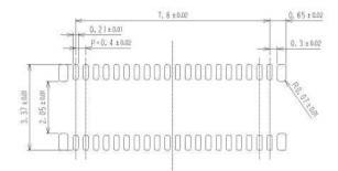
Recommended soldering paste amount: 0.0121 mm<sup>3</sup> (Per 1 Pad)
