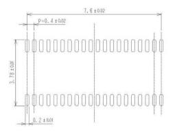
Recommended soldering paste amount: 0.0135 mm<sup>3</sup> (Per 1 Pad)
