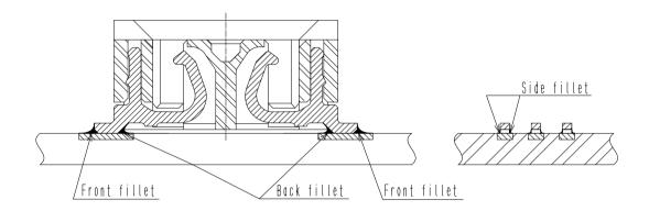
Recommended condition is that fillet thickness is one third of contact thickness (0.13 mm) or more, and solder is wetted completely.
