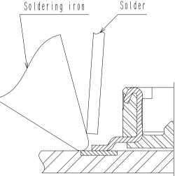
It may affect on mating that the soldering paste height is 0.17 mm of more from the upper surface of the plug contact.
