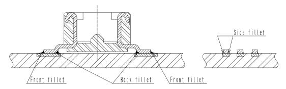
Recommended condition is that fillet thickness is one third of contact thickness (0.13 mm) or more, and solder is wetted completely.
