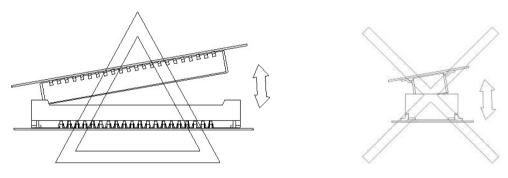
3) Check the rigidity of the FPC for unmating operation prior to your production, otherwise solder breakage and/or connector breakage may occur during unmating process. Lift up the corner of the FPC could apply over stress to the contacts.
