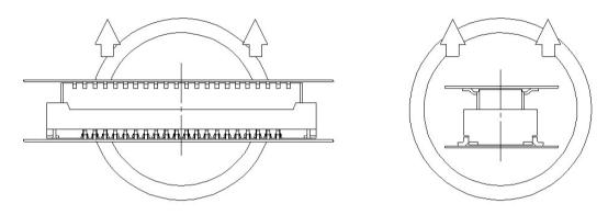
When vertical removal is difficult, lift up either side of longitudinal, contact pitch direction. Do not unmate the connector in connector width direction otherwise the contacts could receive great stress.
