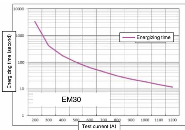
Note : The continuous energizing current graph is reference data used for current values exceeding the rated values for a short time.
