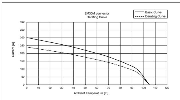
**Operation below the derating curve (dotted line) is recommended.**
