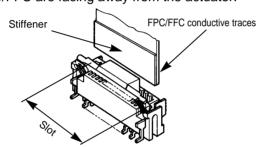
3) Press down the actuator in the direction shown.
