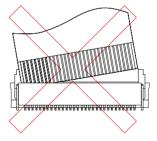
4) Do not press down vertically on the actuator when the FPC/FFC already inserted, it needs to be rotated to engage the lock. Refer to the diagram below. Doing so may cause actuator failure.
