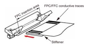
3) Rotate down the actuator until firmly closed. It is critical that the inserted FPC/FFC is not moved and remains fully inserted. Should the FPC/FFC be moved, open the actuator and repeat the process, starting with Step 1 above.
