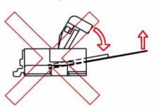
8) At the time of lock operation, application of force such as that indicated by the arrows in the diagrams below will cause the lock lever to disengage. When the lock lever has become disengaged, please exchange the entire con-
