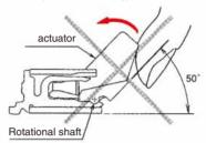
2) Avoid further pressing of the lock portion from the locked condition when the FPC/FFC has not yet been inserted. Doing so will cause the lock lever to become disengaged from the rotational shaft, and the hook portion of the connector body will be damaged.
