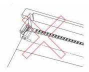
7) When locking, handle the FPC/FFC so that a load is not applied to the FPC/FFC as would occur by pulling the FPC/FFC, or lifting it, etc. When a load is applied in the opposite direction to the rotational movement of the lock, an excessive load will be applied and this will cause connector damage.
