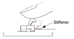
6) Partial insertion of the FPC/FFC, offset insertion, and diagonal insertion will result in an unfavorable engagement of the lock lever in which the lock lever is raised. To correct this, first remove
