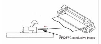
1) Avoid grasping the actuator with two fingers or lifting the actuator with fingernail.
