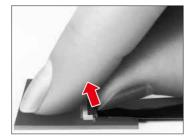
Do not apply excessive force or use any type of tool to operate the actuator.
