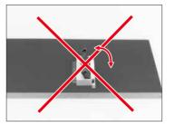
3) Insert the FPC/FFC straight into the insertion opening. Failing to follow this precaution can lead to damaging the FPC/FFC and altering its connectivity.
