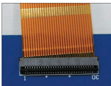
✗ Skewed FPC Insertion
