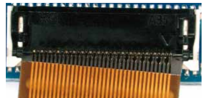
FPC is inserted diagonally.
