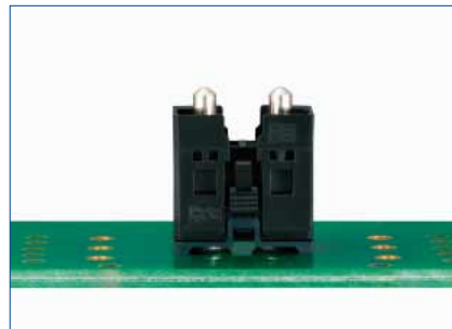
③ Interposer Installed
