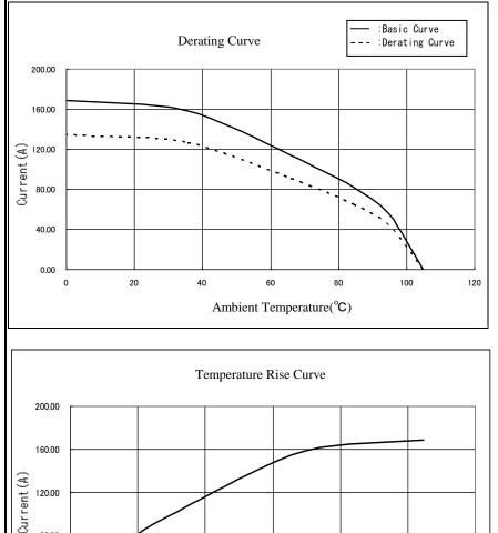
6) The derating curve is derived from the basic curve multiplied by the derating factor of 0.8.7) The value of rated current varies with the ambient temperature. It is recommended to use the product within the derating curve zone.
