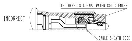
ANTI-LOOSENING SOLVENT IS UNNECESSARY FOR THE INITIAL ASSEMBLY. FOR REASSEMBLY. TO TREAT POSSIBLE MISWIRING. IT IS RECOMMENDED THAT HENKEL JAPAN Ltd., LOCTITE 263 AND LOCTITE PRIMER 7649 BE APPLIED TO THE MALE THREADS OF BOTH THE J HOUSING AND THE HOOD.
