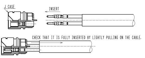
CHECK THE WIRING AFTER INSERTING THE CONTACTS.
