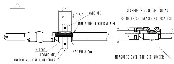
TABLE. 3 CRIMP STRENGTH (WITH RECOMMENDED TOOL) THERE SHOULD BE NO REMOVAL OR LOOSENING OF THE CABLE WHEN THE CABLE IS PULLED WITH A FORCE LESS THAN THOSE SHOWN BELOW. ! IF THE HEIGHT IS WRONG, PLEASE CHECK THE TOOL.
