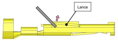
② Lift up the lance to the extent that the tip protrudes slightly (approximately half of the plate thickness) over the lance protection wall.
