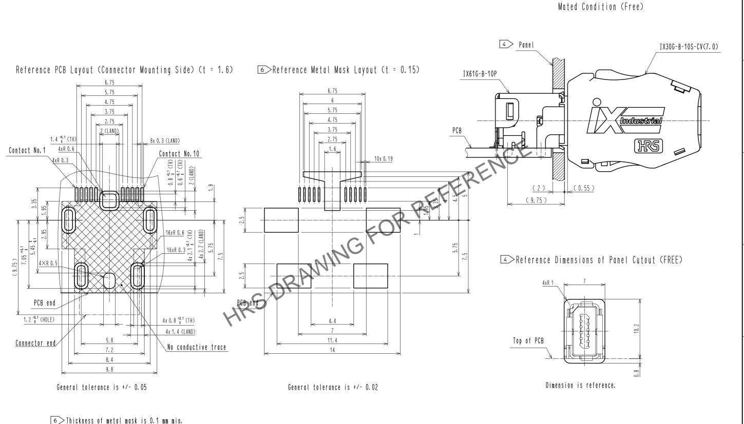
Metal mask dimensions of the drawings described, are reference dimensions for 0.15 mm thickness metal mask.
