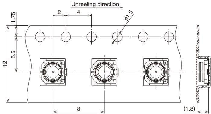
The above diagram shows the embossed carrier tape dimensions used to package D.FL75-R-SMT-1(40).
