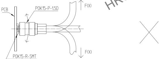
\* If you use this product without the fixing structure, If the force acts in the direction differently from the center of the product, it may cause the loss of function due to eccentricity of the product.
