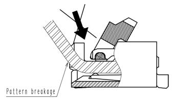
◆Checking the Locking Condition
