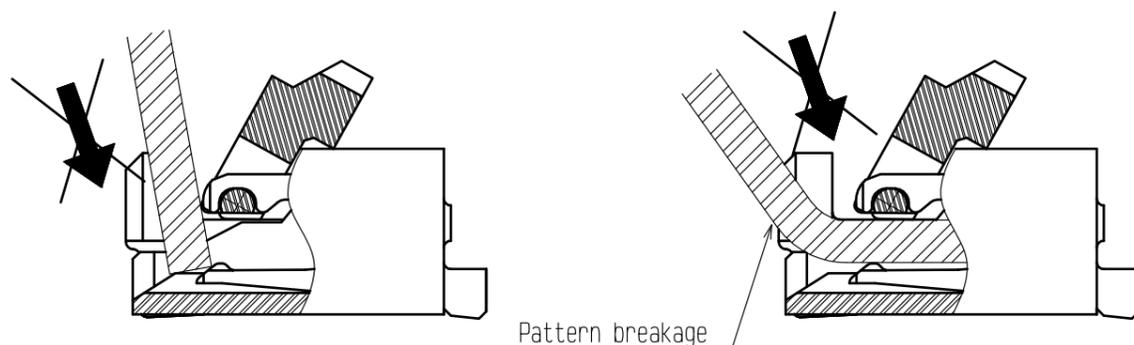
◆Checking the Locking Condition
