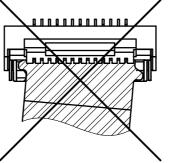
When FPC TAB is on right or left guide for positioning FPC, it causes the loose connection.
