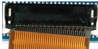
FPC is inserted diagonally.
