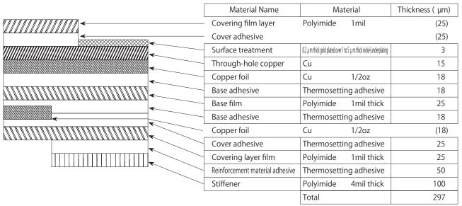
Note: To prevent release of the FPC due to bending, use of double-sided FPC with copper foil on the back side is not recommended.
