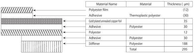
Note : Typical thickness tolerance is about  $\pm$  20  $\mu$  m
