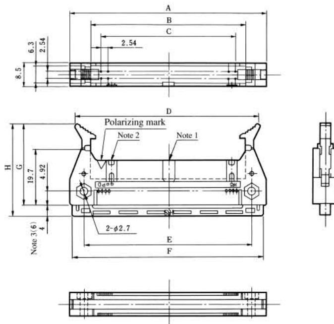
Note 1, Note 2 : The number of polarizing slot and key installed positions changes according to products.
