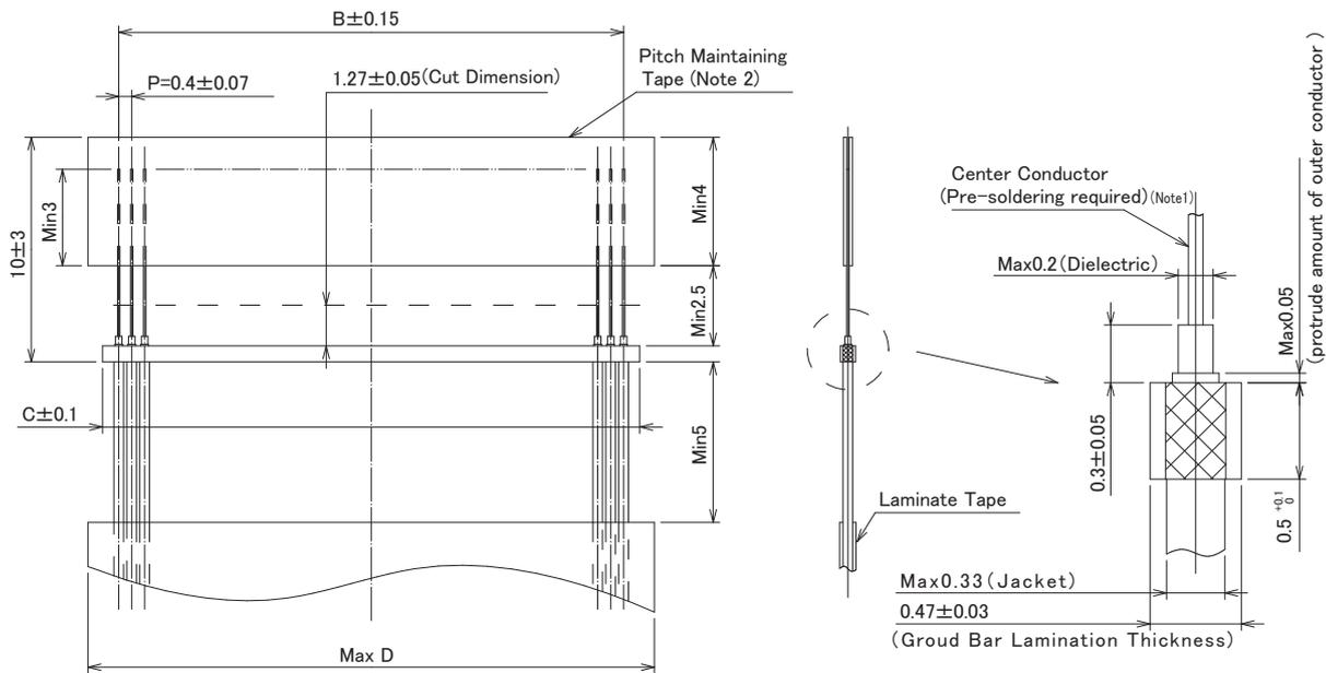
Note 1 : Center conductor requires pre-soldering (lead-free).
