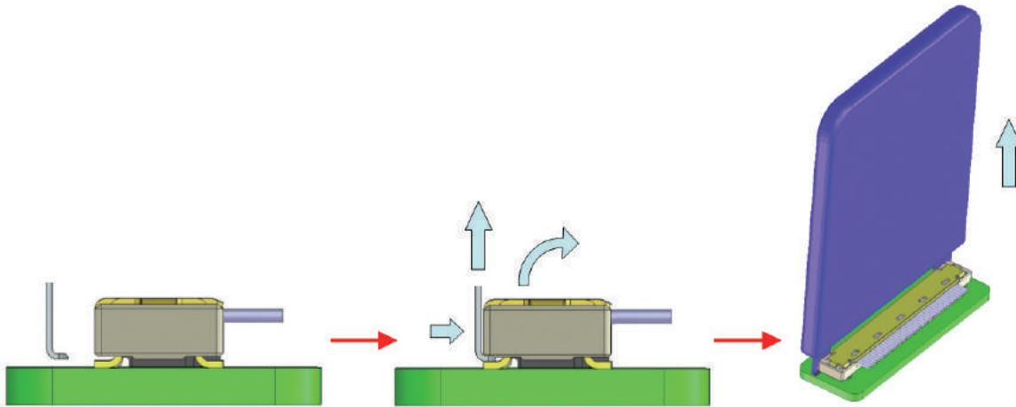
Note 1 : Do not mate / unmate the connectors when receptacle is not mounted on the board.
