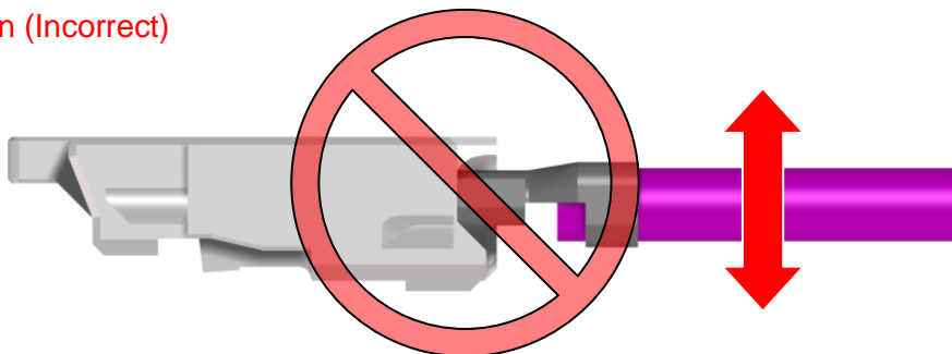
Twisted insertion (incorrect)
