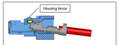
If inserted diagonally(upward), the housing lance may be damaged
