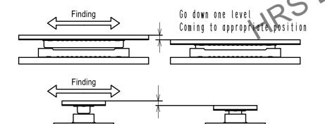
(2) When quiding, the connectors are aligned parallel to each other, with longitudinal and lateral movements restricted. Mate them properly by applying force in this condition.
