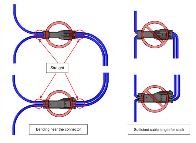
Fig.8 Image of wiring
