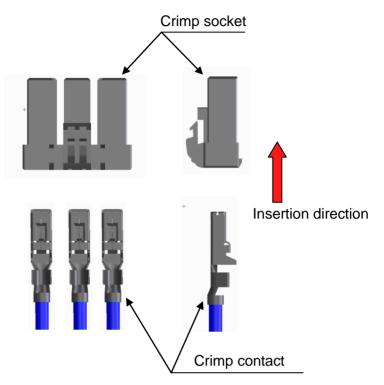
How to insert wire into multipole contact
