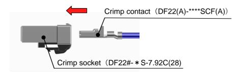
Insert the contact in a horizontal direction to the crimp socket. Please insert the contact at once until you hear click sound and feeling.
