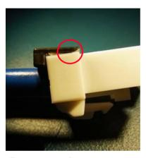
· Front edge of the retainer is touching to the crimp housing.
