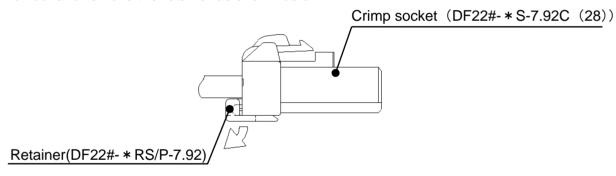
• By doing repair, the retainer lock strength could be lower, therefore, do not reuse the retainer, and replace it to a new one.
