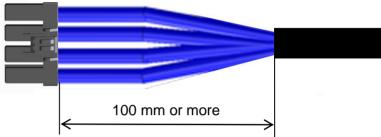
When using a multipole terminal, be aware that the strip length for the outside cables should be longer to provide it with a flection portion, as well as to not apply any load such as excessive torsion.
