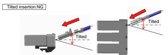
Insertion with tilted angle may deform the contact or crimp socket. Please Insert the contact without tilted.
