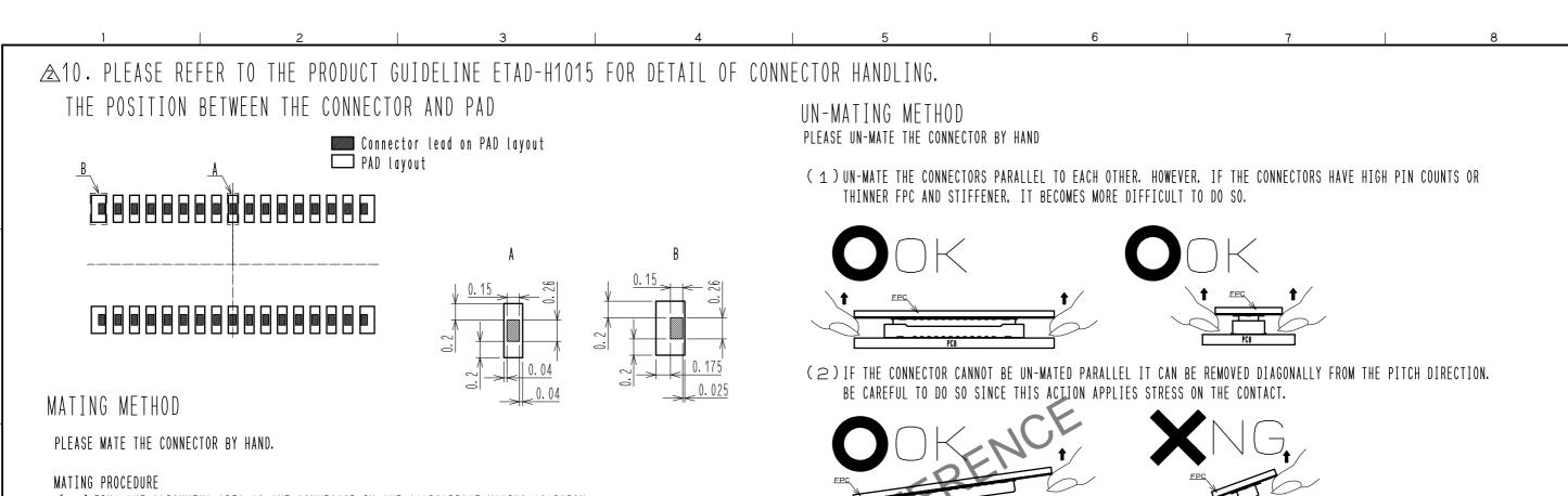
(1) FIND THE ALIGNMENT AREA TO THE CONNECTOR IN THE APPROPRIATE MATING POSITION. THIS CONNECTOR HAS AN ALIGNMENT CHAMBER(GUIDANCE RIBS) ON RECEPTACLE SIDE AND 'R' ON PLUG SIDE.
