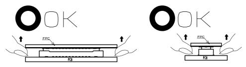
UN-MATED PARALLEL IT CAN BE REMOVED DIAGONALLY FROM THE PITCH DIRECTION.
