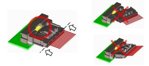
When connecting, make sure that the receptacle and plug are combined correctly.
