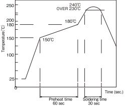
Recommended Reflow Conditions Temperature Profile (Connector Top Surface)
