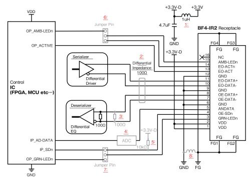
Receptacle Connection Example (Internal Board Connection)
