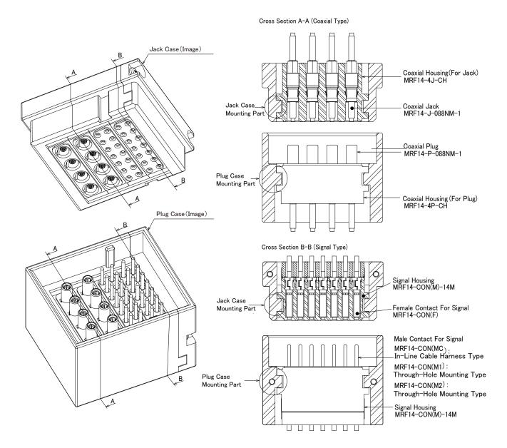
Note: Lock and guide pin are purchased separately. Contact a Hirose sales representative for installation details and dimensions.
