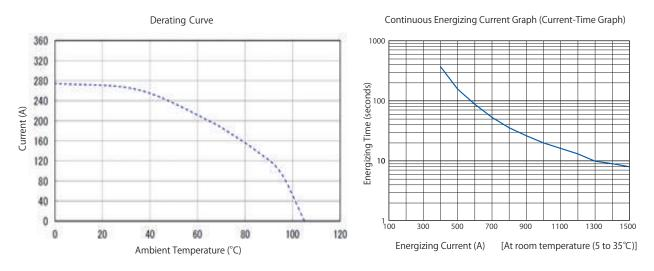
Operation below the derating curve (dotted line) is recommended.
