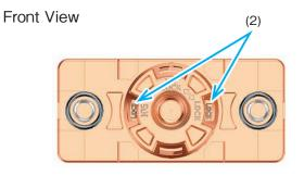
(3) The position marks shown of the plug and the receptacle match with each other.Plug position markCircular concave shapeReceptacle position markRectangular concave shape
