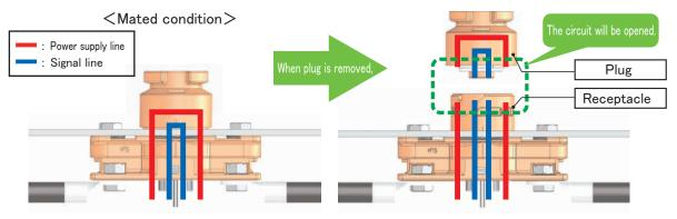
When the connector is unmated, the circuit is physically disconnected, ensuring the safety of workers.
