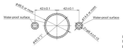
Recommended panel thickness t=2 to 4.5mm Ensure that the surface roughness of the waterproof surface is  $\sqrt{Rz3.2}$ .
