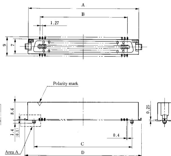
Note : The connector positioning bosses are constructed to press fit into the board with light force. When mounting on the board, press the connector lightly from the top and check that the positioning bosses are securely inserted in the board holes and that the connector leads are engaged in the board. The recommended boss hole for use with automatic mounting is illustrated in fig. 1.
