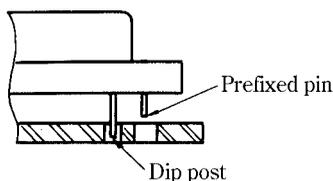
Note : In order to prevent the dip post breakage in the connector installation to the board, please insert the board in parallel to the connector so that the prefixed pin may be forcibly pushed in, after the dip post is guided to the board through-hole.
