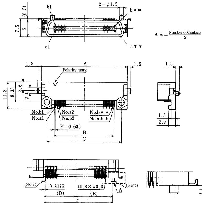
Note : The FX2A type does not have bosses as shown in the illustration.
