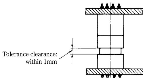
Set the tolerance clearance within 1mm to mate the male and female connectors.
