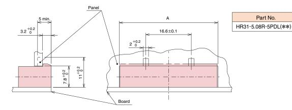
1.2 Recommended mounting panel dimensions (straight through hole type)
